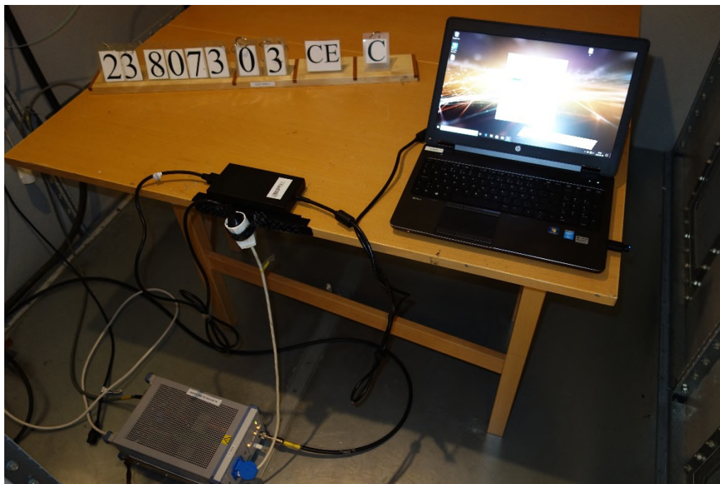
Test setup picture in Conducted Emission chamber
