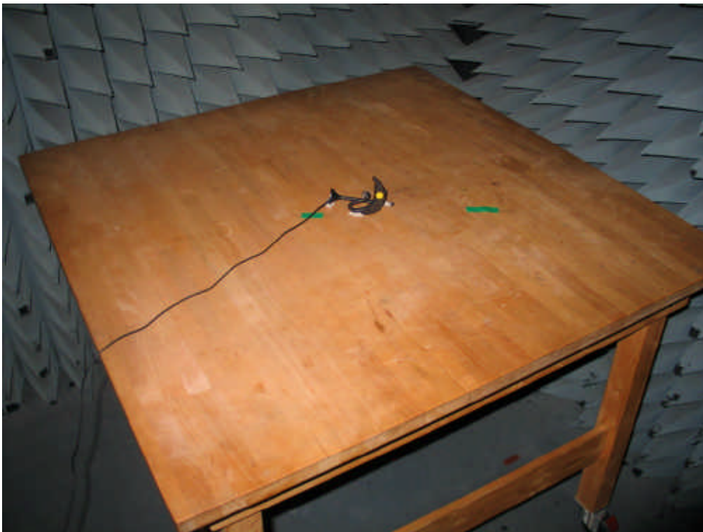
Photo 2: Test setup for radiated measurements (Enclosure, below 30 MHz)
