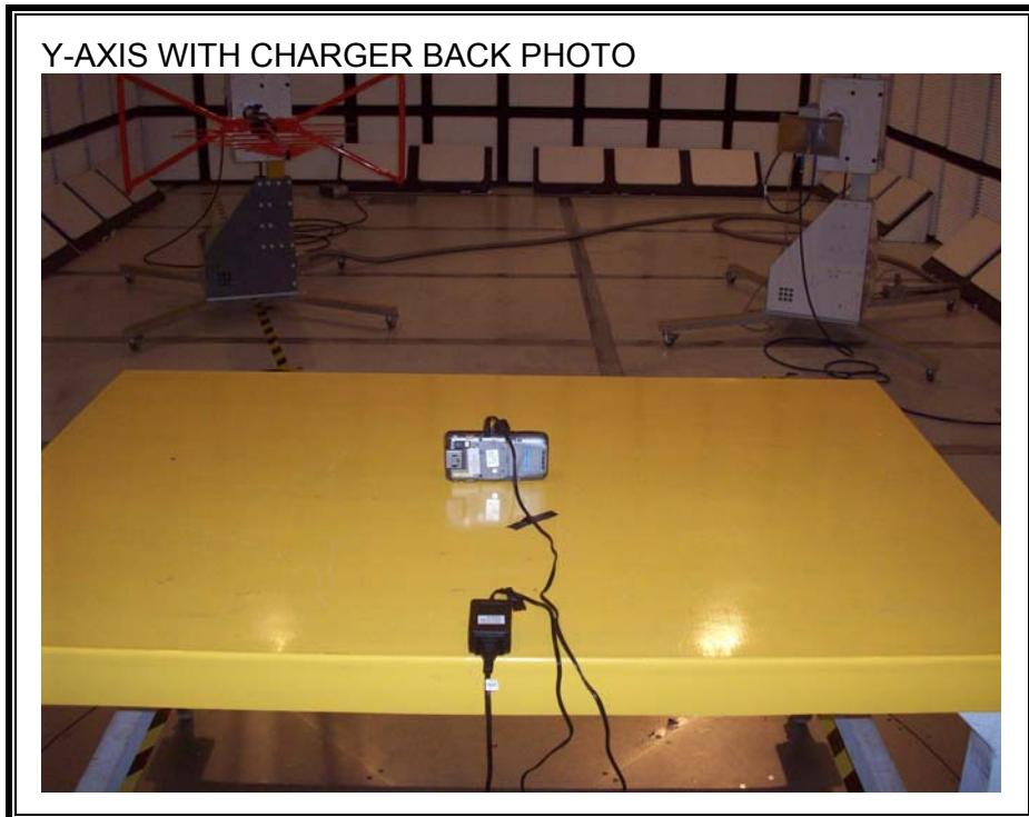
**POWERLINE CONDUCTED EMISSIONS MEASUREMENT SETUP**
