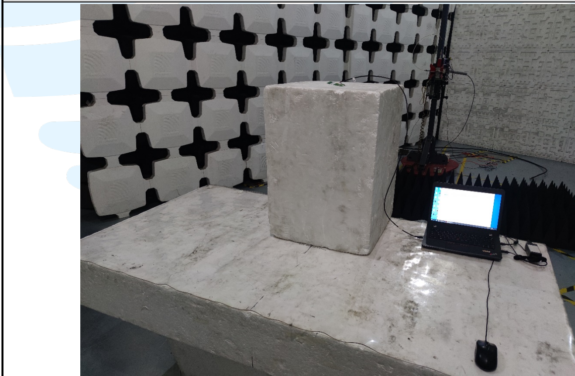
Radiated emission Test Setup (Above 1 GHz)
