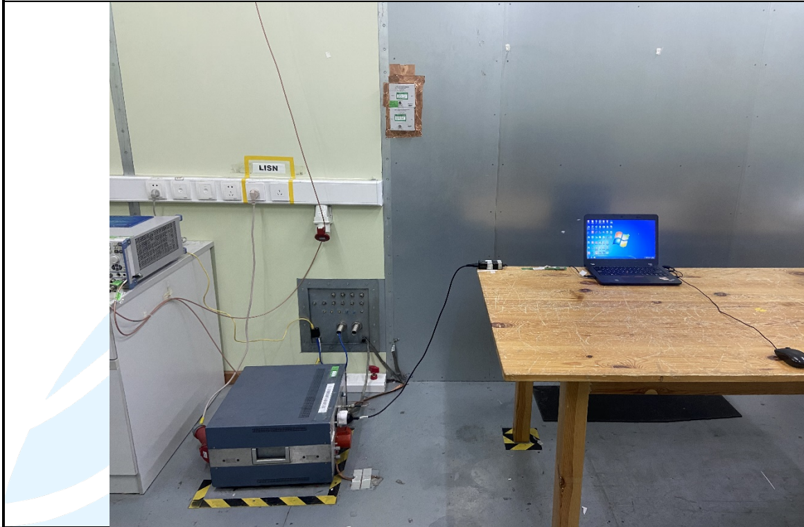
Conducted Emission Test Setup
