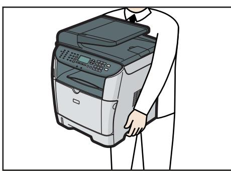
7. There are three upright pins on the optional paper feed unit. Align them with the holes on the underside of the machine, and then carefully lower the machine onto them.
