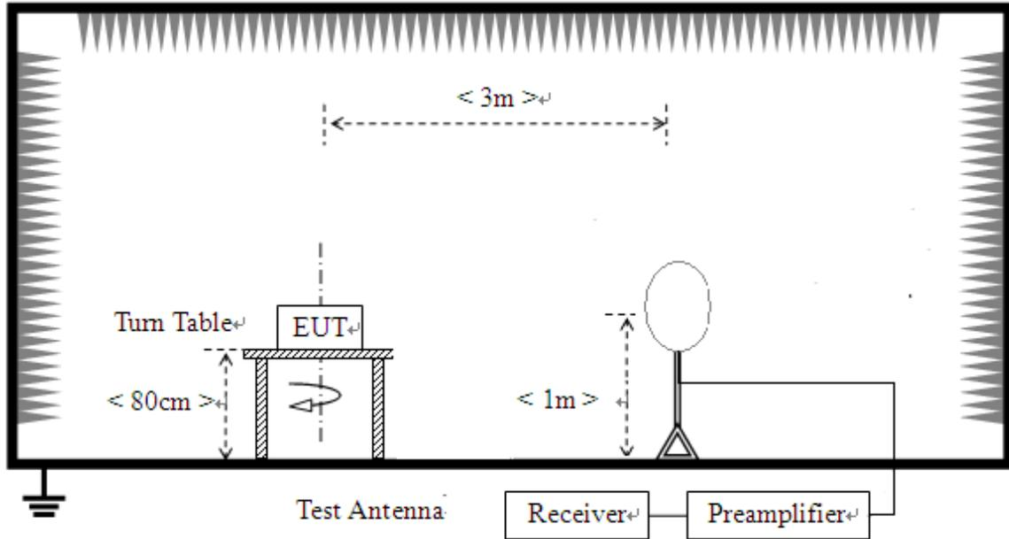
For radiated emissions from 30MHz to 1GHz
