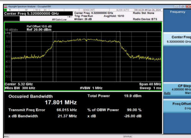
U-NII-2a 99% & 26dB Bandwidth-802.11n(20MHz) ,5320MHz,Ant1
