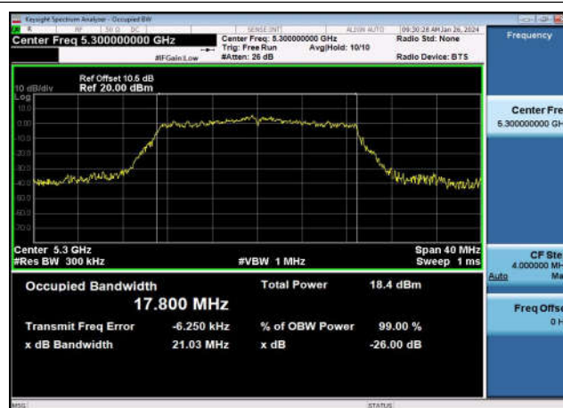
U-NII-2a 99% & 26dB Bandwidth-802.11ac(20MHz) ,5300MHz,Ant1
