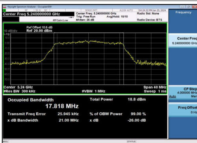
U-NII-1 99% & 26dB Bandwidth-802.11ac(20MHz) ,5240MHz,Ant1
