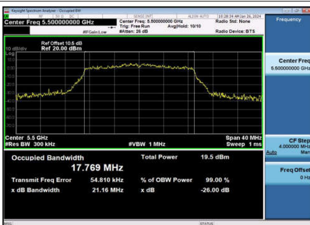
U-NII-2c 99% & 26dB Bandwidth-802.11n(20MHz),5500MHz,Ant1
