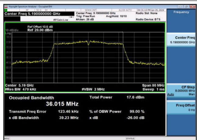
U-NII-1 99% & 26dB Bandwidth-802.11ac(40MHz) ,5190MHz,Ant1
