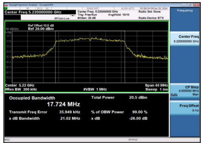
U-NII-1 99% & 26dB Bandwidth-802.11n(40MHz) ,5190MHz,Ant1
