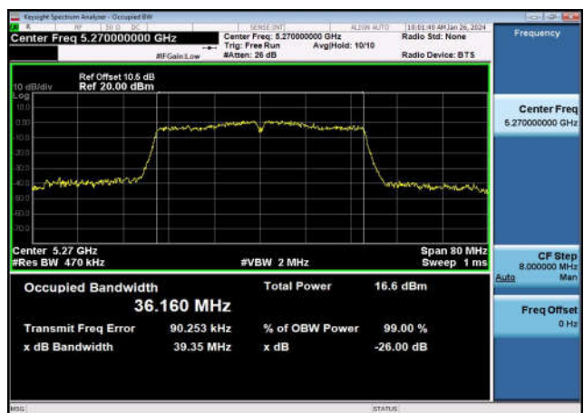
U-NII-2a 99% & 26dB Bandwidth-802.11ac(80MHz),5290MHz,Ant1
