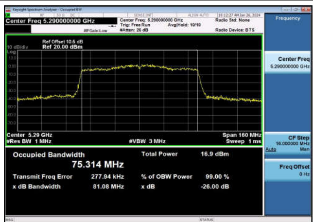
U-NII-2c 99% & 26dB Bandwidth-802.11n(20MHz),5580MHz,Ant1
