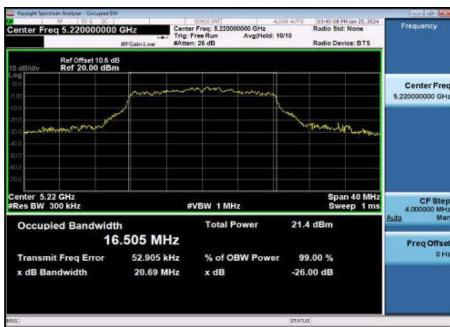
U-NII-1 99% & 26dB Bandwidth-802.11ac(20MHz) ,5180MHz,Ant1
