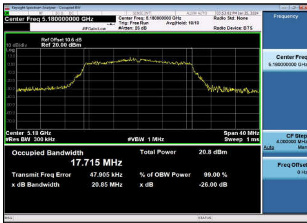
U-NII-1 99% & 26dB Bandwidth-802.11n(20MHz) ,5240MHz,Ant1
