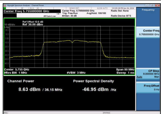
U-NII-3 Output Power-802.11ac(80MHz) ,5775MHz,Ant1
