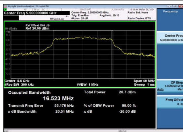
U-NII-2c 99% & 26dB Bandwidth-802.11a(20MHz) ,5500MHz,Ant1
