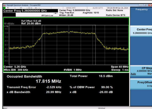
U-NII-2a 99% & 26dB Bandwidth-802.11ac(20MHz) ,5260MHz,Ant1
