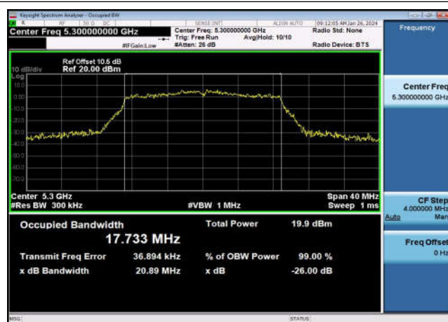
U-NII-2a 99% & 26dB Bandwidth-802.11n(40MHz) ,5270MHz,Ant1
