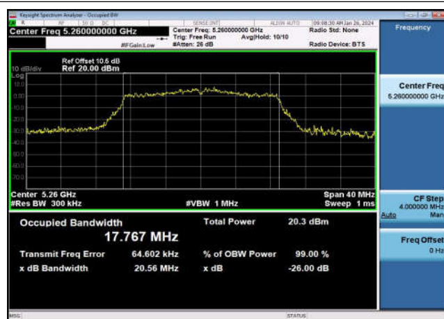
U-NII-2a 99% & 26dB Bandwidth-802.11n(20MHz) ,5320MHz,Ant1
