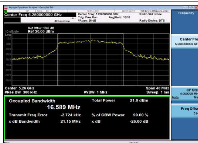
U-NII-2a 99% & 26dB Bandwidth-802.11a(20MHz) ,5320MHz,Ant1
