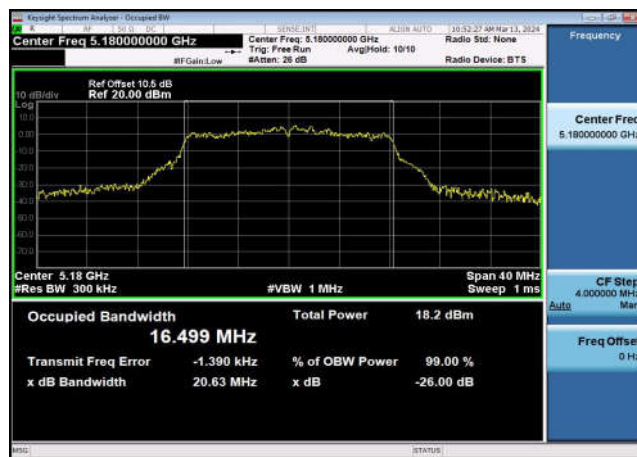
U-NII-1 99% & 26dB Bandwidth-802.11a(20MHz) ,5180MHz,Ant1
