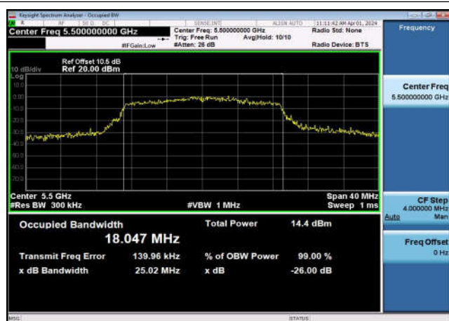
U-NII-2c 99% & 26dB Bandwidth-802.11n(20MHz),5500MHz,Ant1
