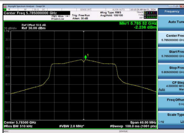
U-NII-3 Power spectral density-802.11 ac(20MHz),5785MHz,Ant1
