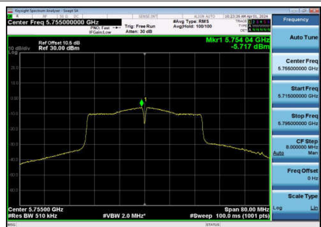
U-NII-3 Power spectral density-802.11 ac(80MHz),5775MHz,Ant1
