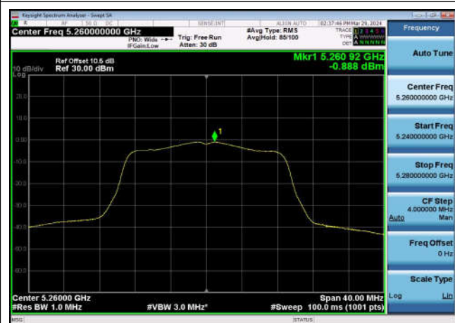
U-NII-2a Power spectral density-802.1 1n(20MHz),5320MHz,Ant1
