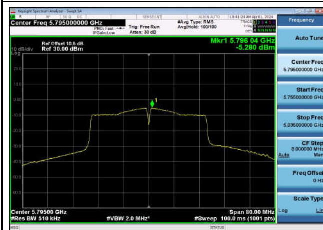
U-NII-3 Power spectral density-802.11 ac(40MHz),5795MHz,Ant1
