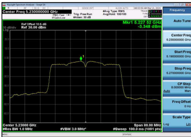
U-NII-1 Power spectral density-802.11 n(40MHz),5230MHz,Ant1
