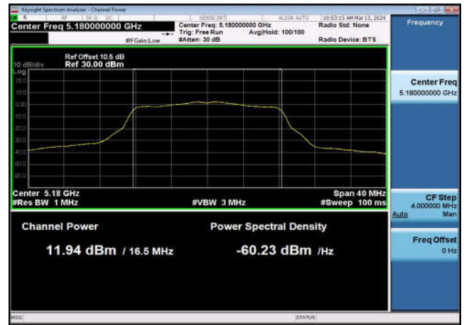
U-NII-1 Output Power-802.11a(20MHz) ,5180MHz,Ant1
