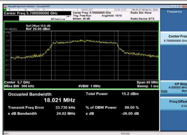
U-NII-2c 99% & 26dB Bandwidth-802.11ac(40MHz) ,5550MHz,Ant1
