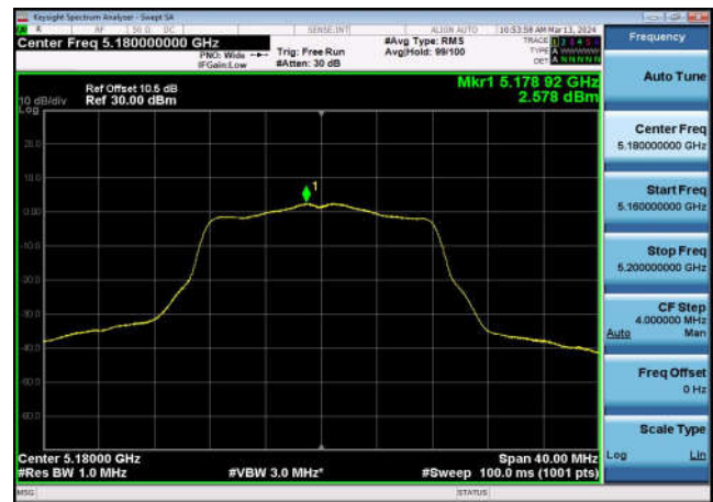
U-NII-1 Power spectral density-802.11 a(20MHz),5180MHz,Ant1
