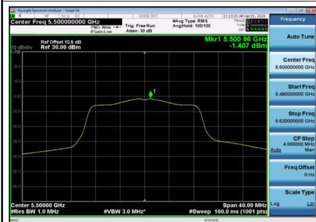
U-NII-2c Power spectral density-802.1 1n(20MHz),5500MHz,Ant1
