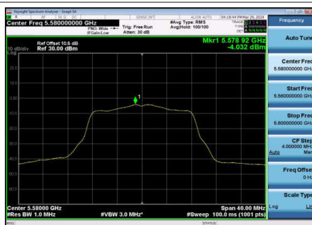
U-NII-2c Power spectral density-802.1 1a(20MHz),5580MHz,Ant1
