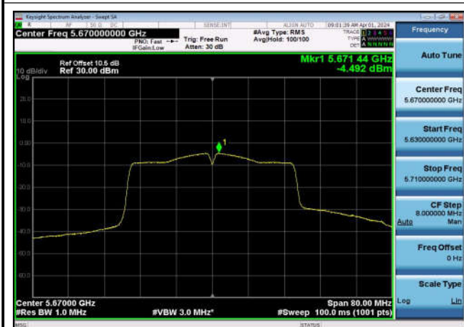
U-NII-3 Power spectral density-802.11 n(20MHz),5745MHz,Ant1
