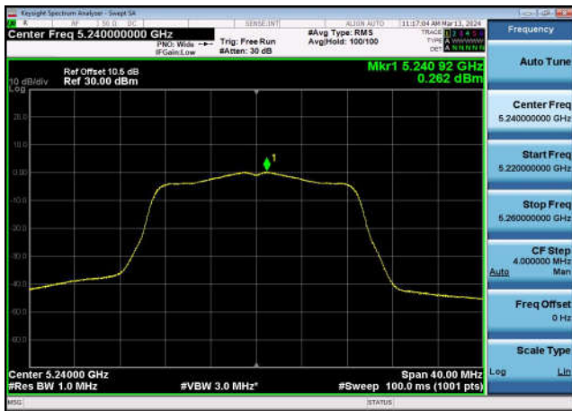
U-NII-1 Power spectral density-802.11 n(40MHz),5230MHz,Ant1
