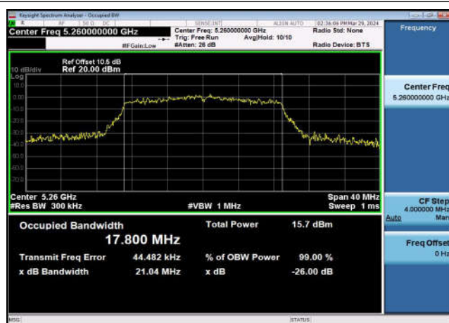
U-NII-2a 99% & 26dB Bandwidth-802.11n(20MHz) ,5320MHz,Ant1
