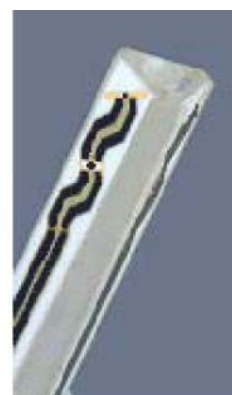
Figure 3.3 Probe Thick-Film Technique
