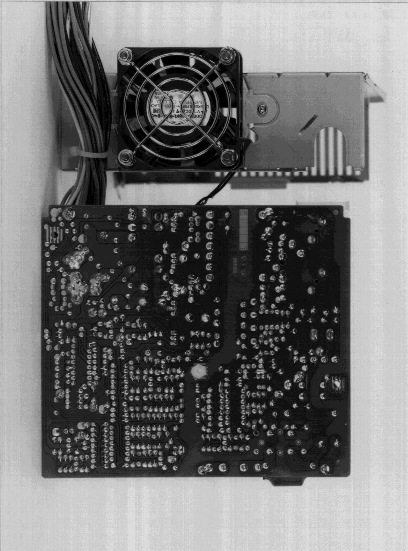
6.4 ASTEC Power supply, Components side
