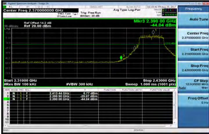
802.11n\_HT20: Band Edges Test Data CH-12
