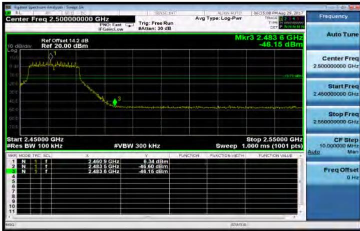
802.11n\_HT20: Band Edges Test Data CH-13
