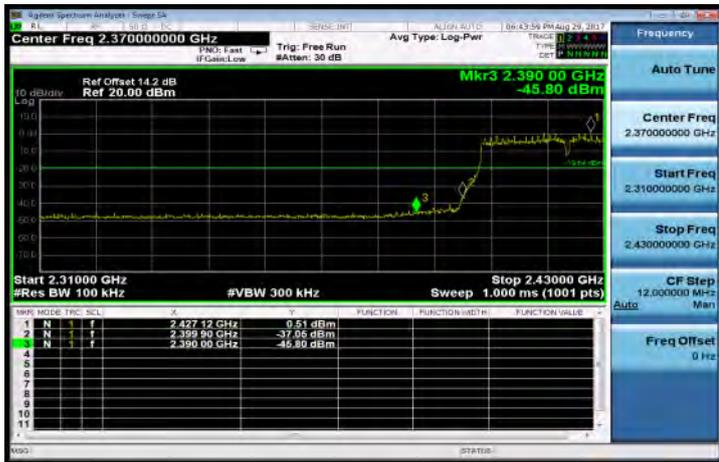
802.11n\_HT40: Band Edges Test Data CH-10
