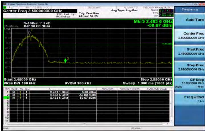
802.11b: Band Edges Test Data CH-13
