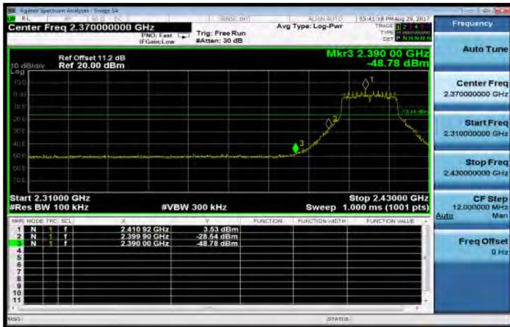
802.11g: Band Edges Test Data CH-12
