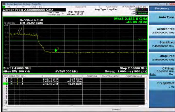
802.11n\_HT40: Band Edges Test Data CH-11
