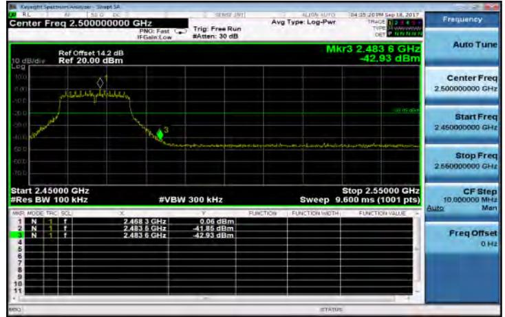
802.11n\_HT20: Band Edges Test Data CH-High
