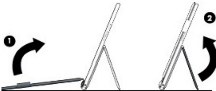
3. Place the softcover on a flat surface, and then pull out the computer to remove it.
