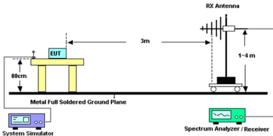
For radiated test above 1GHz
