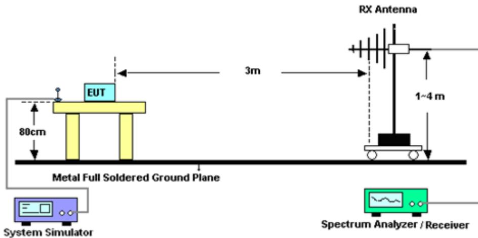
For radiated test from 1GHz to 18GHz
