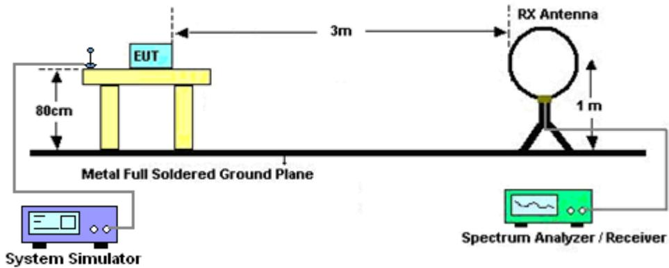
For radiated emissions from 30MHz to 1GHz
