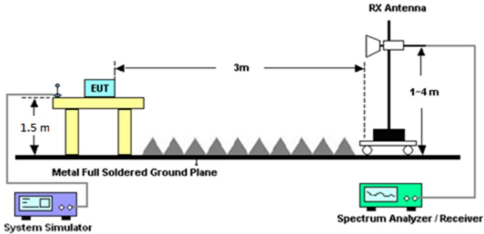
For radiated test above 18GHz
