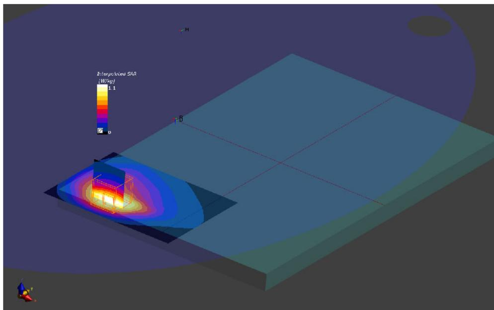
**9. LTE Band 30, QPSK - 10MHz, CH27710, Back face position**
