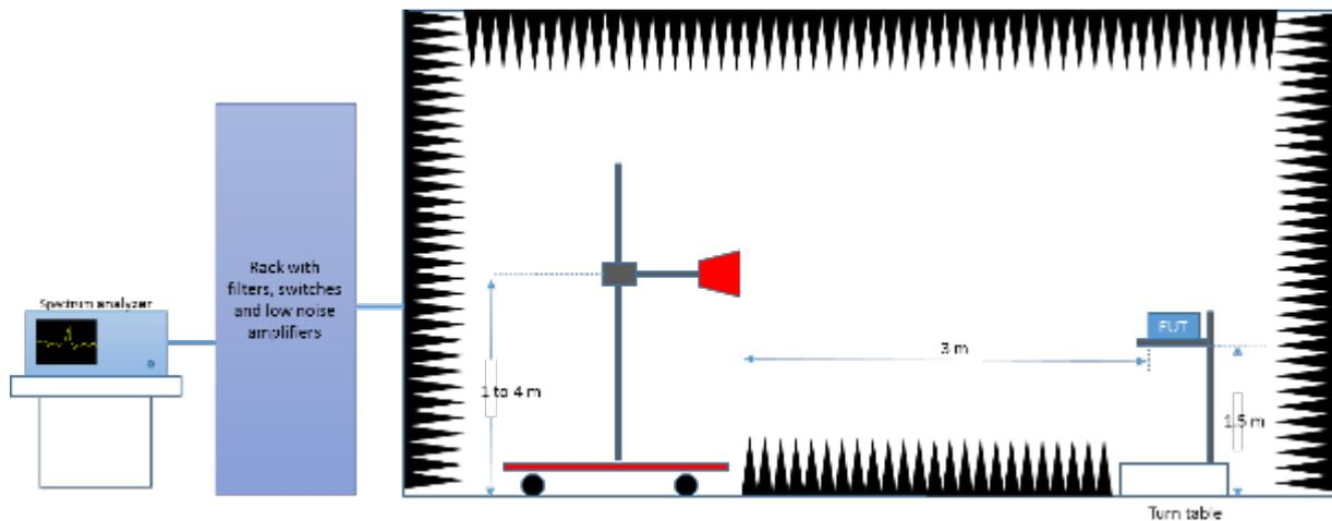
*Radiated Setup Frequency range 18 GHz to 26.5 GHz*
