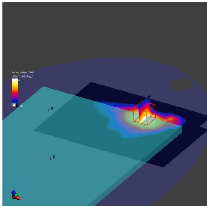
**5. LTE Band 5, 1RB Mid @ QPSK - 10MHz, CH20525 , Main Antenna – Back Face**
