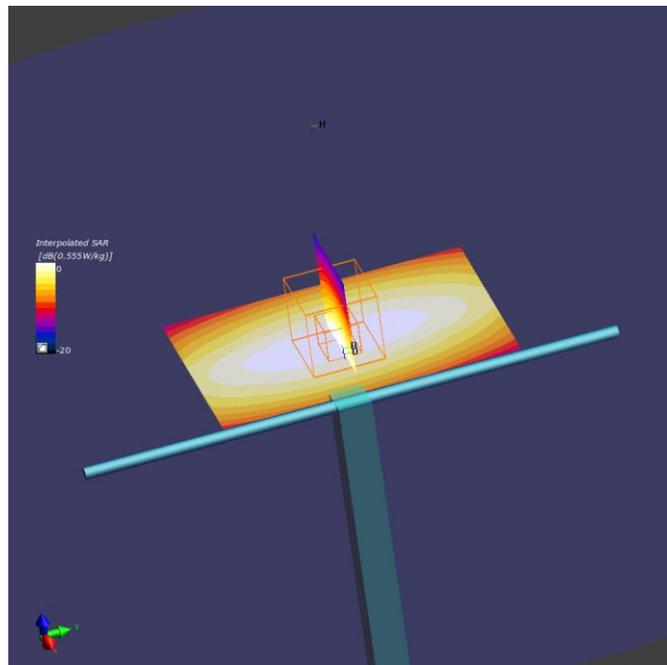
**16. System Check Body Liquid 835MHz – 2019-12-31**
