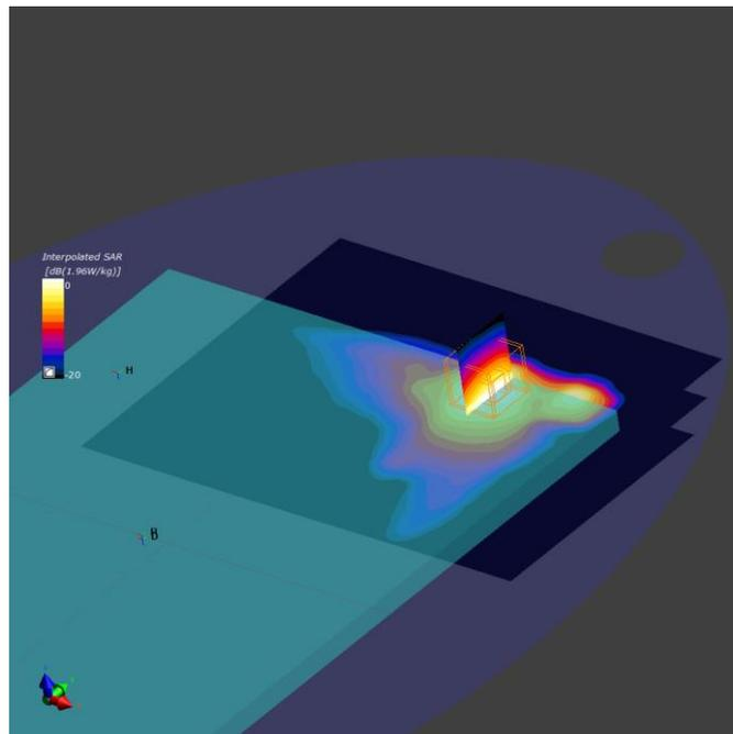
**13. LTE Band 66, 50RB Mid @ QPSK - 20MHz, CH132072 , Main Antenna – Laptop**
