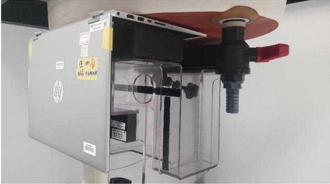
A photograph showing the laptop mode of the test setup. A silver laptop is open and placed inside the transparent test chamber. A black and red probe is positioned above the laptop. The chamber is mounted on a stand. |
