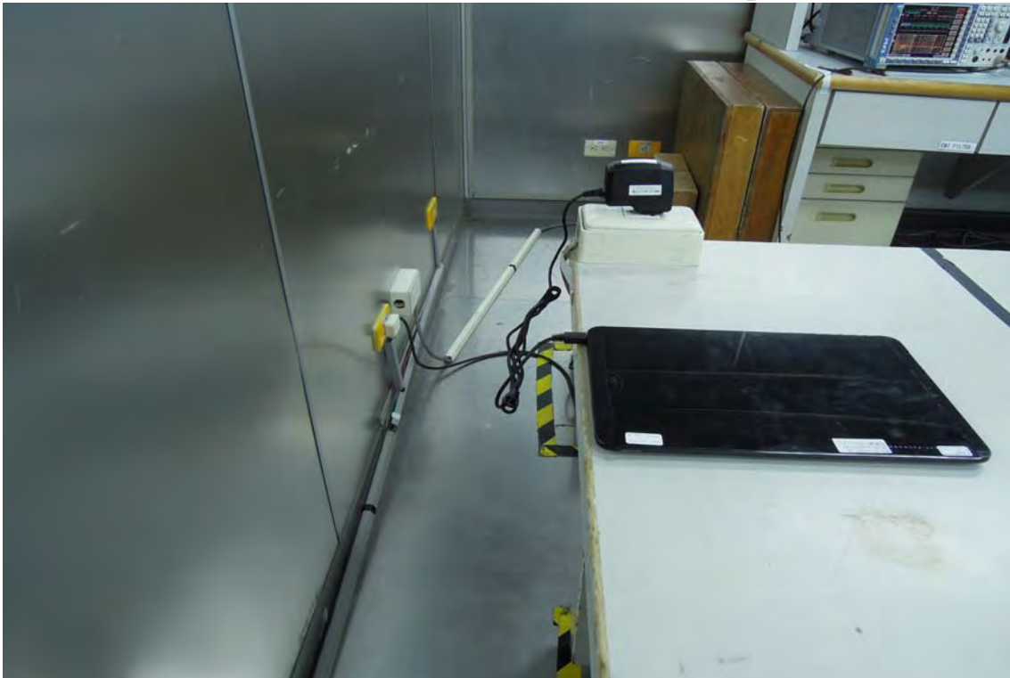
AC Power-line Conducted Emission Set up Photo
