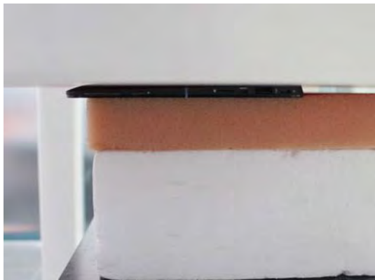
Fig.3 Back side to flat phantom
