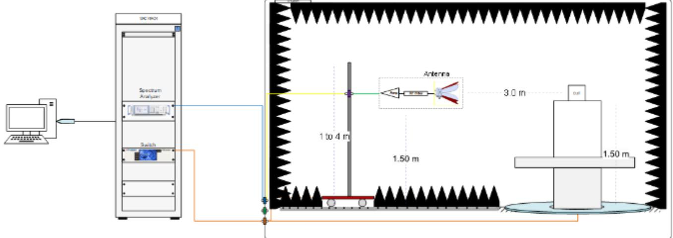
Radiated Setup 18 GHz – 40 GHz (Transmitter tests)
