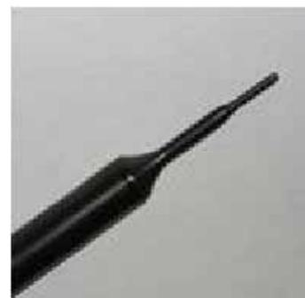
Figure 4.4 EX3DV4 E-field Probe
