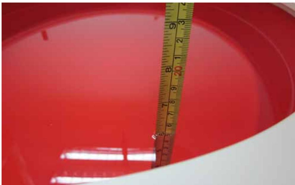
Figure 4.4: Liquid depth in the Flat Phantom
