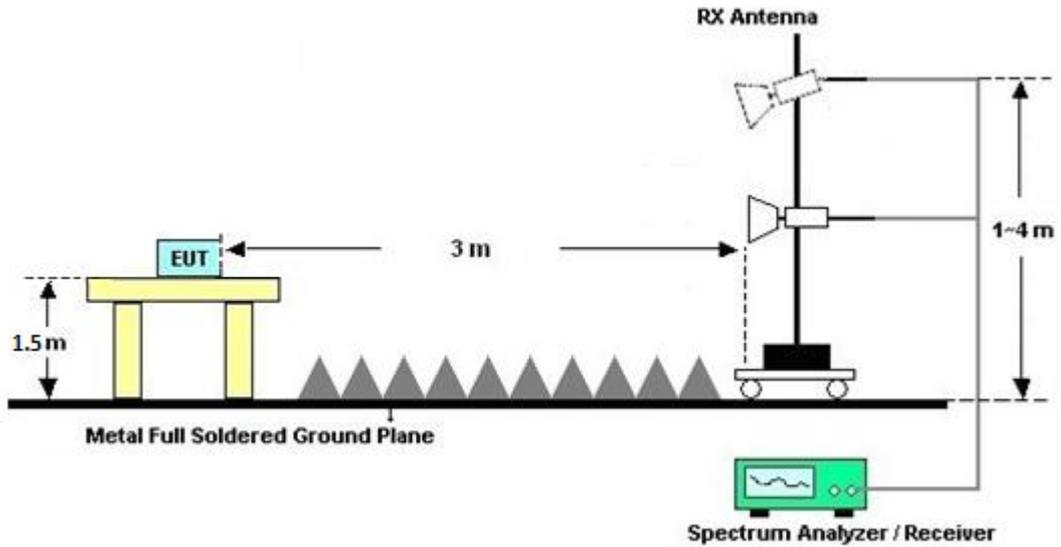
For radiated test above 18GHz
