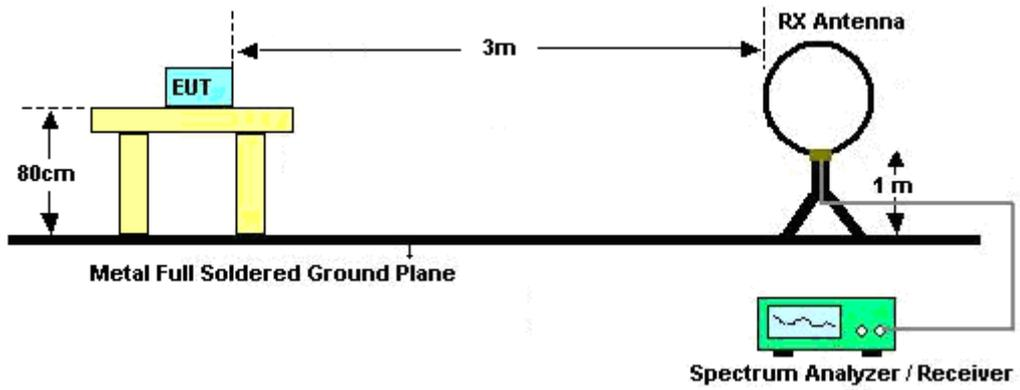
For radiated test from 30MHz to 1GHz
