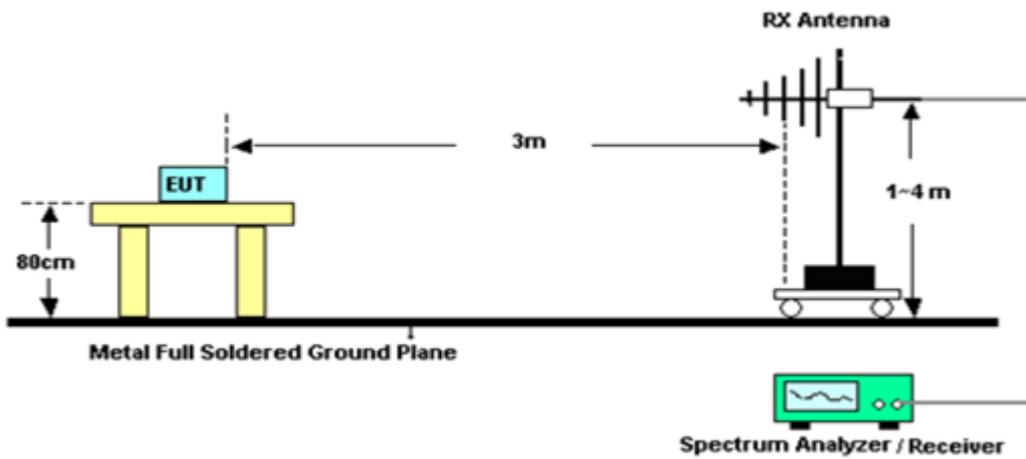
For radiated test from 1GHz to 18GHz
