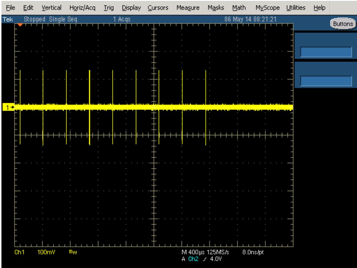
Figure 8 FCC Type 6 Radar (9 pulses in each burst)
