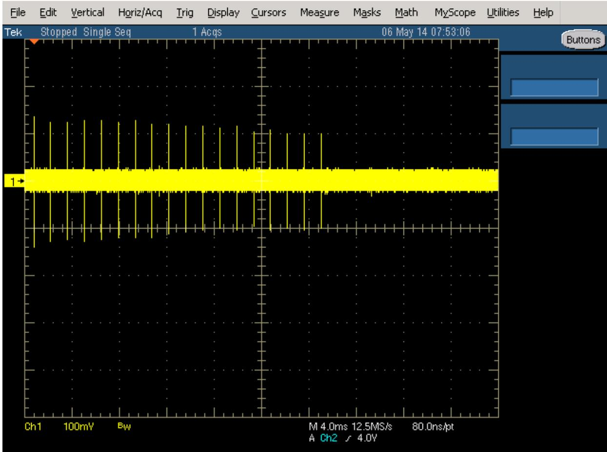
**Figure 3 FCC Type 1 Radar (18 pulses)**
