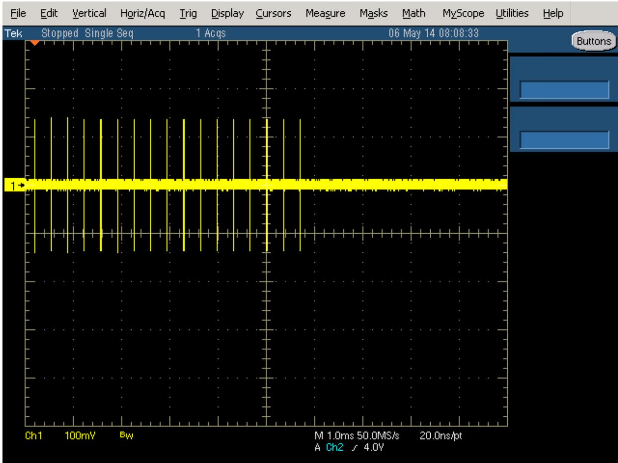
Figure 5 FCC Type 3 Radar (17 pulses)
