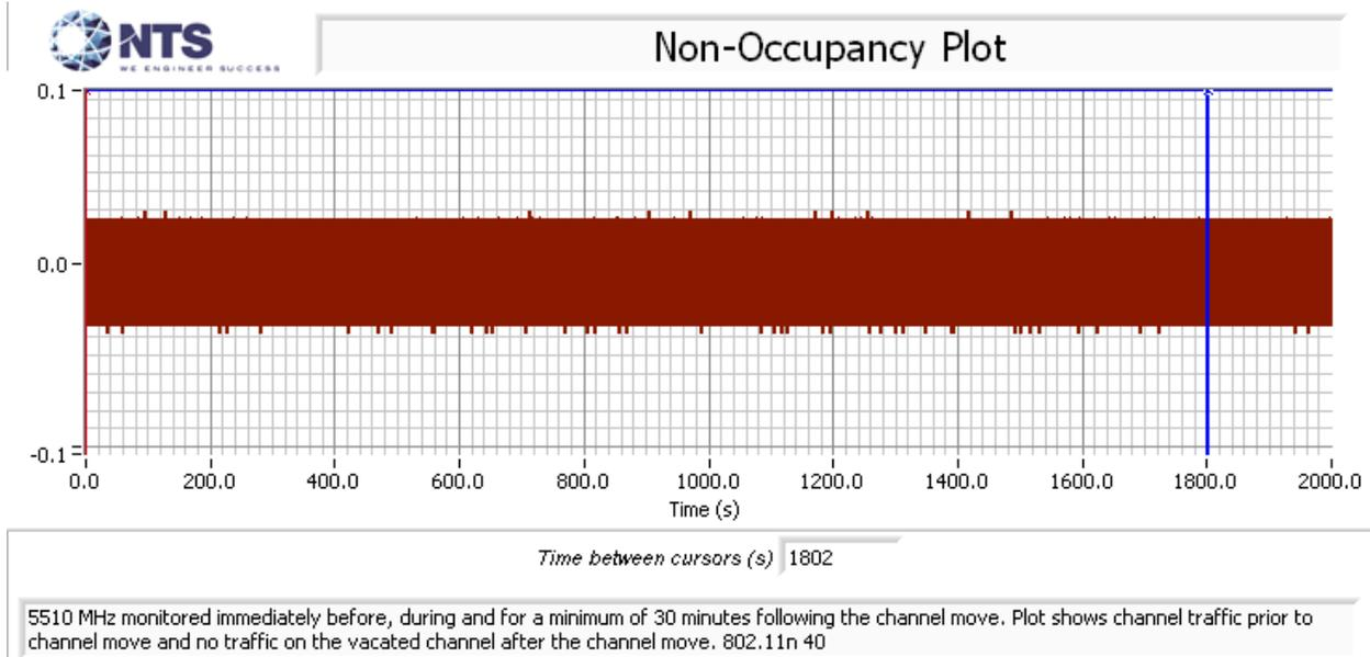
**Figure 12 Radar Channel Non-Occupancy Plot (n40 mode)**
