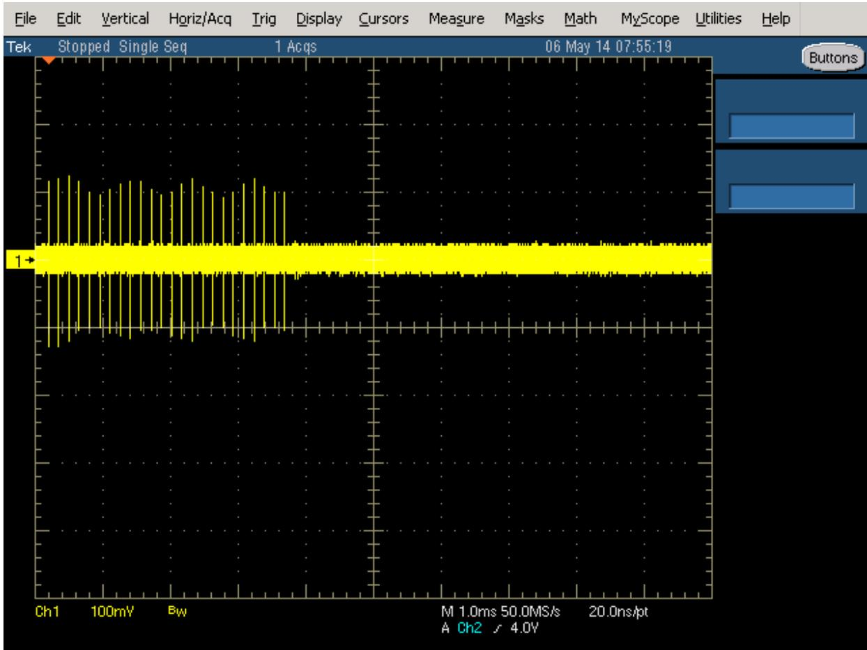
Figure 4 FCC Type 2 Radar (24 pulses)
