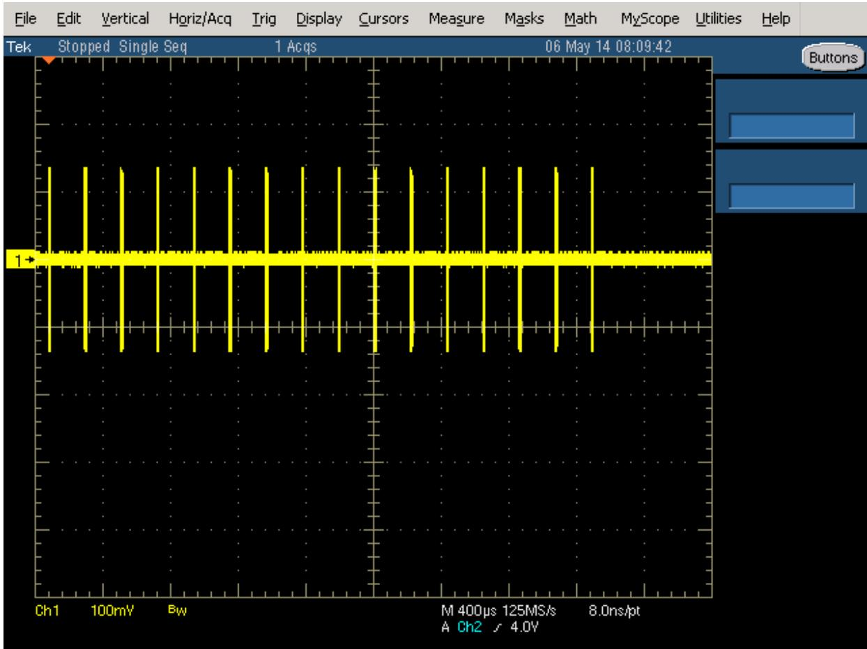
Figure 6 FCC Type 4 Radar (16 pulses)
