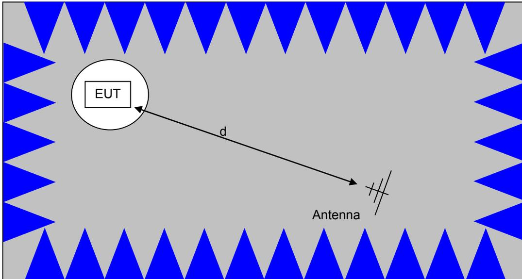
The anechoic materials on the walls and ceiling ensure compliance with the normalized site attenuation requirements of CISPR 16 / CISPR 22 / ANSI C63.4 for an alternate test site at the measurement distances used.
