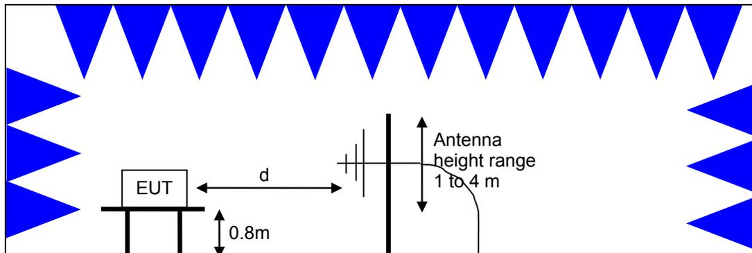
Test Configuration for Radiated Field Strength Measurements
