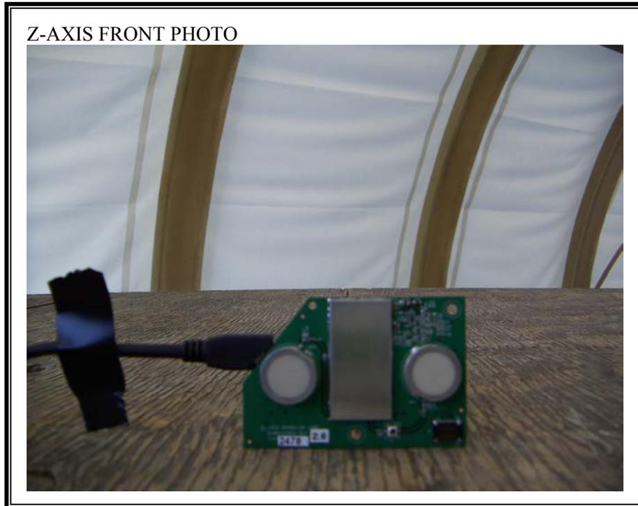
**DIGITAL DEVICE RADIATED EMISSIONS SETUP (USB 1.1)**
