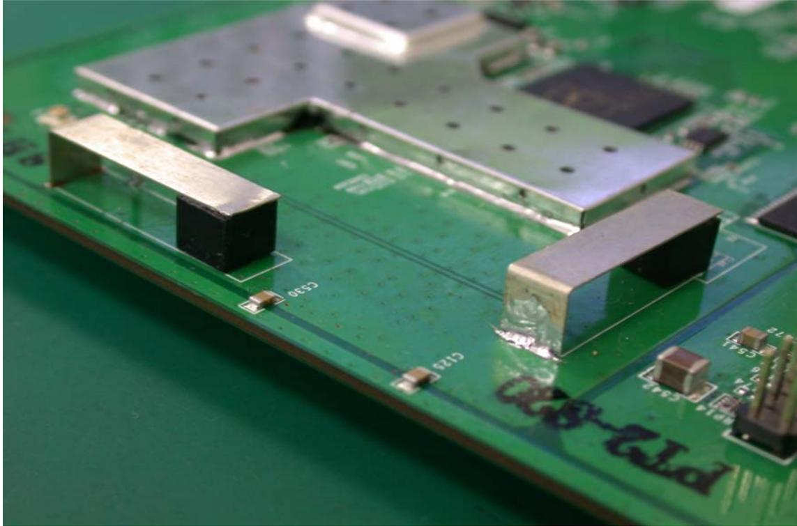
**Antenna 10 / 11: INTERNAL PIFA Antenna / 4.9 ~ 5.9GHz / 5.95dBi**
