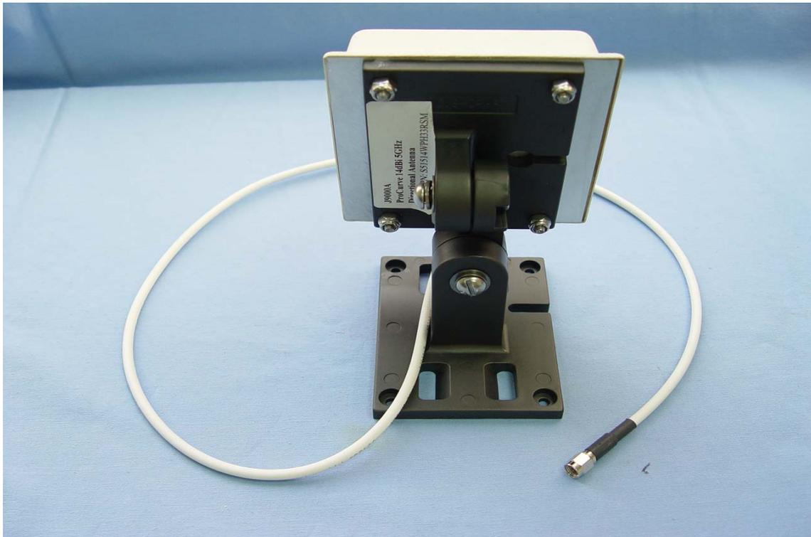
**Antenna 8 / 9: INTERNAL PIFA Antenna / 2.4 ~ 2.5GHz / 5.92dBi**
