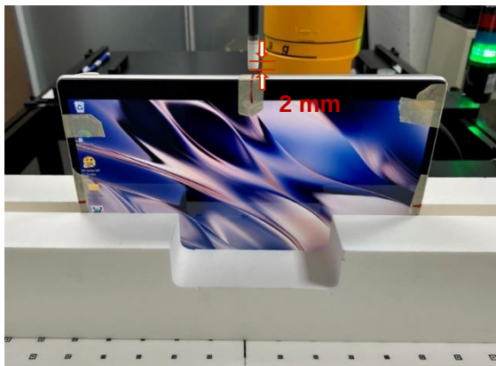
Photograph 9. PD, Top Edge, 2mm
