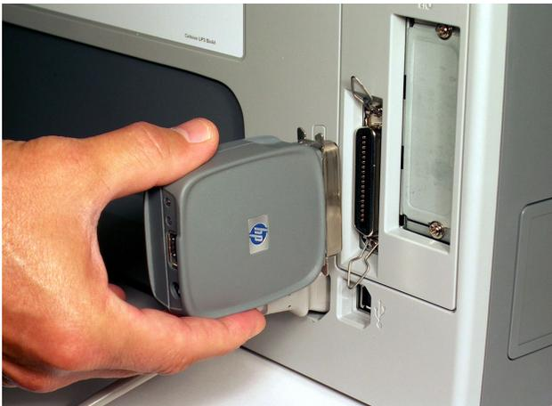
Installing the hp bt1300 onto the parallel port
