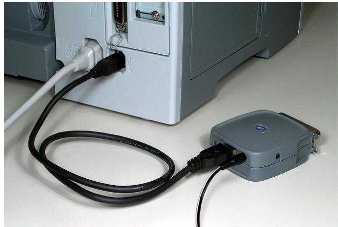
Installing the hp bt1300 using the USB connection
