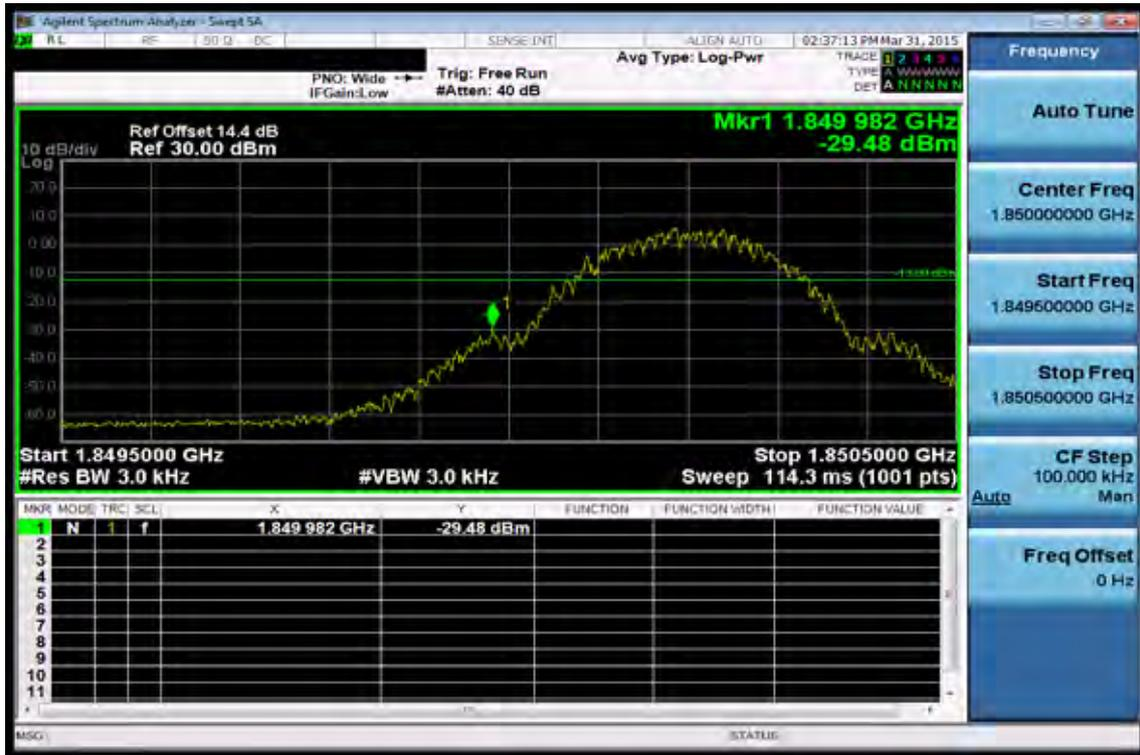
**Band edge emission at antenna terminals – GPRS 1900 Channel Highest**
