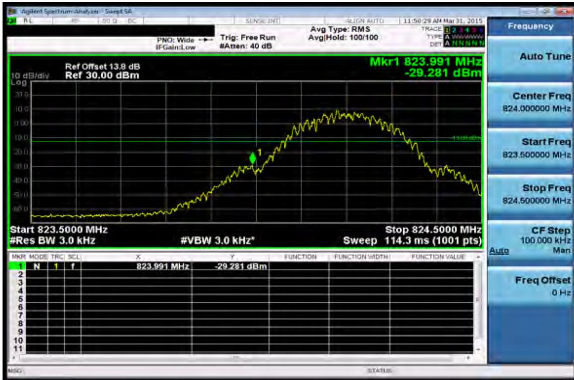
**Band edge emission at antenna terminals – GPRS 850 Channel Highest**
