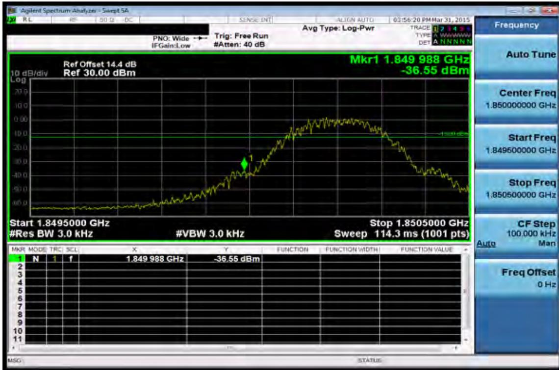
**Band edge emission at antenna terminals – EDGE 1900 Channel Highest**
