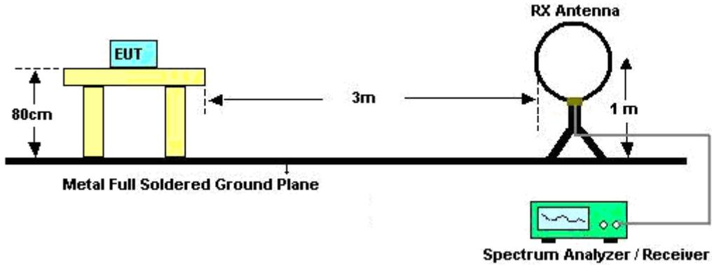
For radiated emissions from 30MHz to 1GHz
