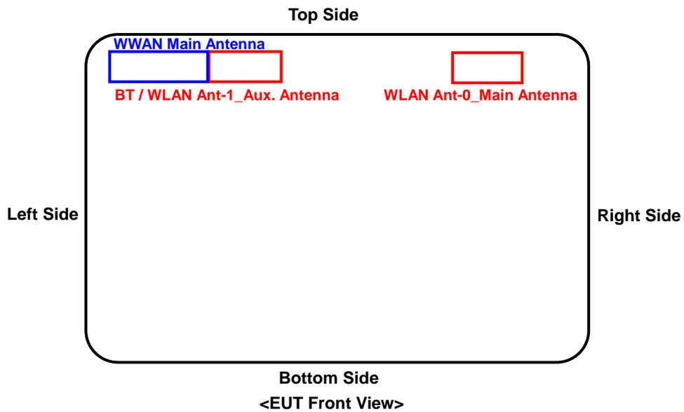
The separation distance for antenna to edge:
