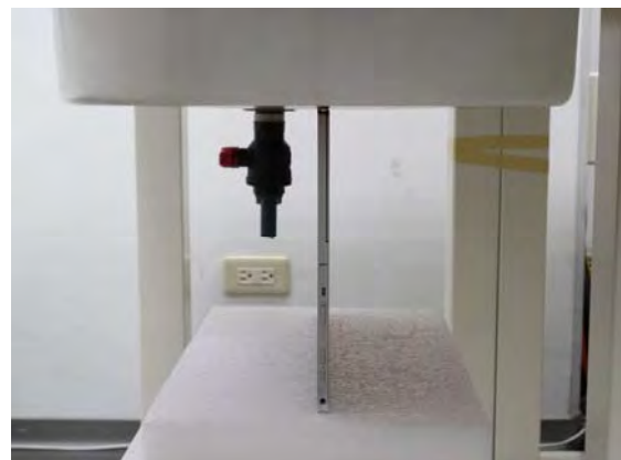
Fig.5 EUT Bottom side to flat phantom
