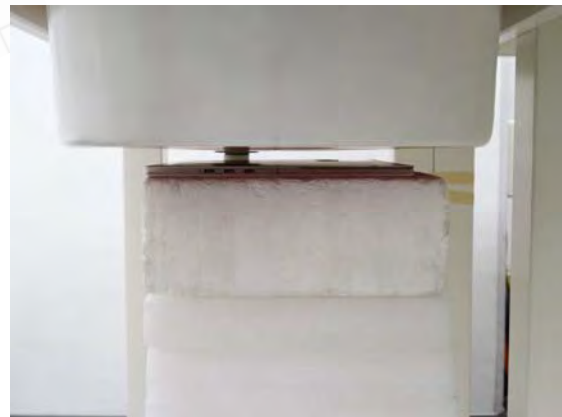
Fig.4 EUT Back side (14mm) to flat phantom
