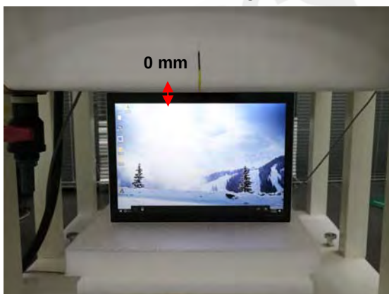
Fig.5 EUT Bottom side to flat phantom
