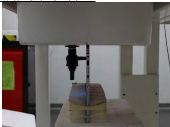
Fig.6 EUT Top side to flat phantom
