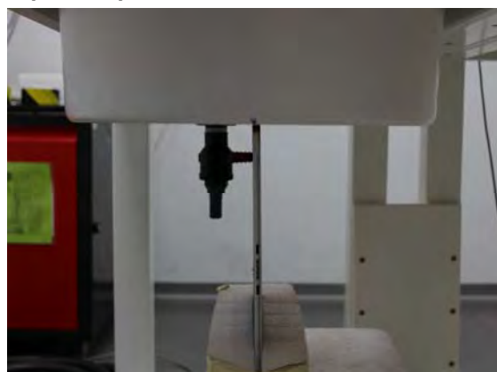
Fig.5 EUT Right side to flat phantom
