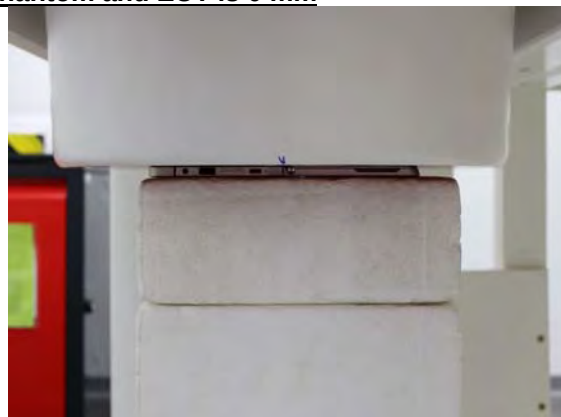
Fig.3 EUT Back side to flat phantom
