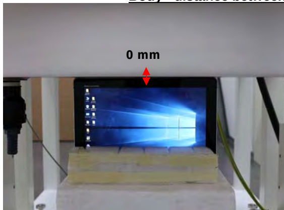
Fig.6 EUT Top side to flat phantom
