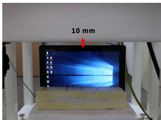
Fig.7 EUT Top side (10mm) to flat phantom
