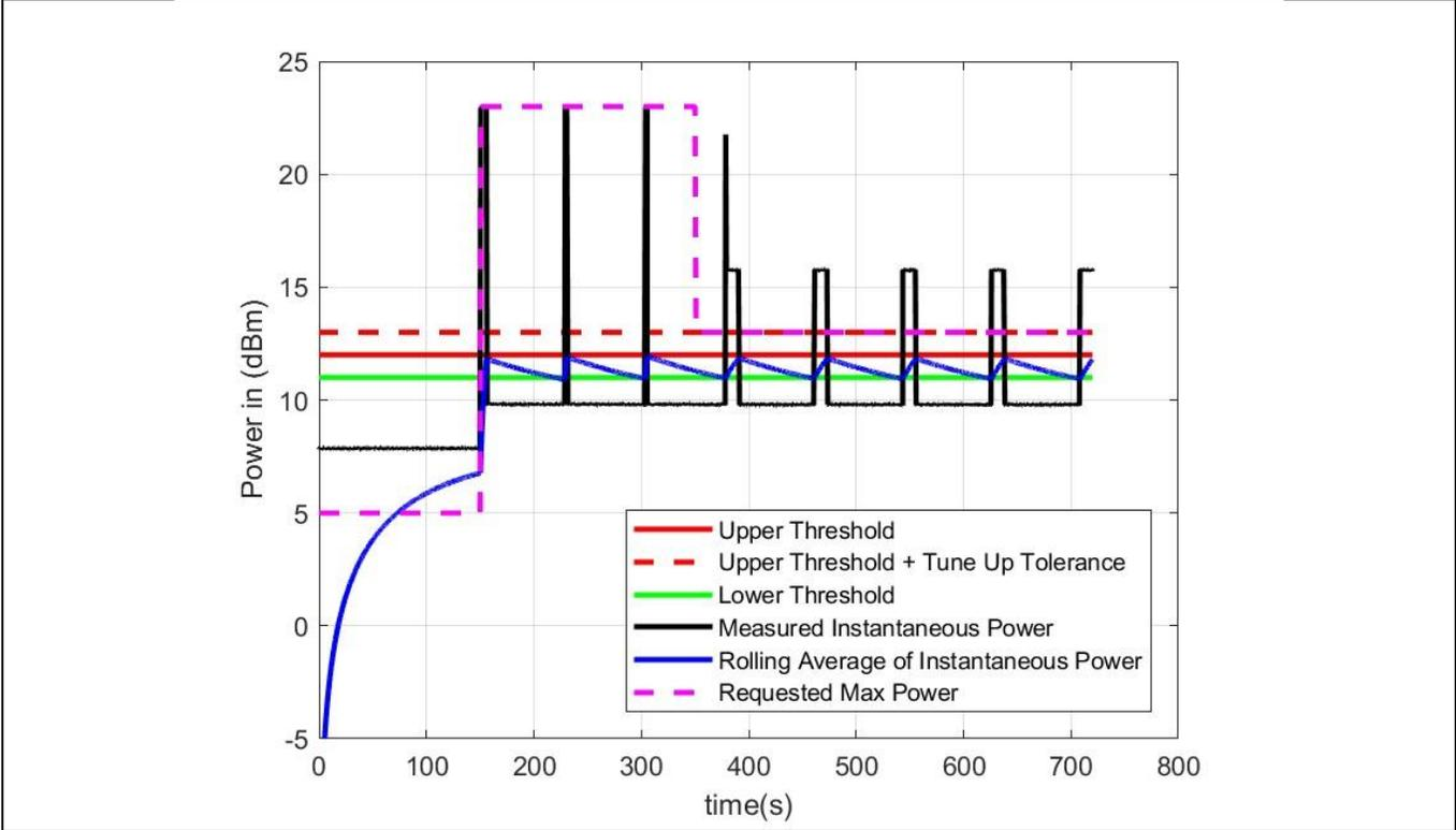
**Case #2: Sequence 2 - LTE Band 2 – Max Power 24 dBm – Roll Period 100 sec – Check Period 0.05 sec**
