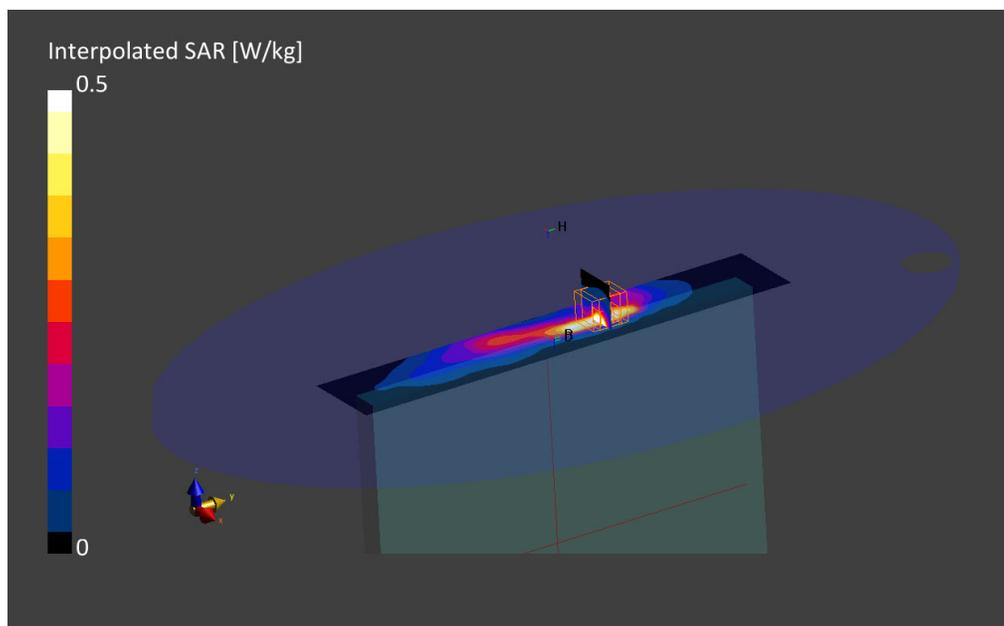
**9. LTE Band 17, QPSK - 10MHz, CH23790, Bottom edge**
