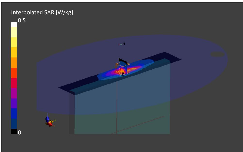
**7. LTE Band 13, QPSK - 10MHz, CH23230, Bottom edge**
