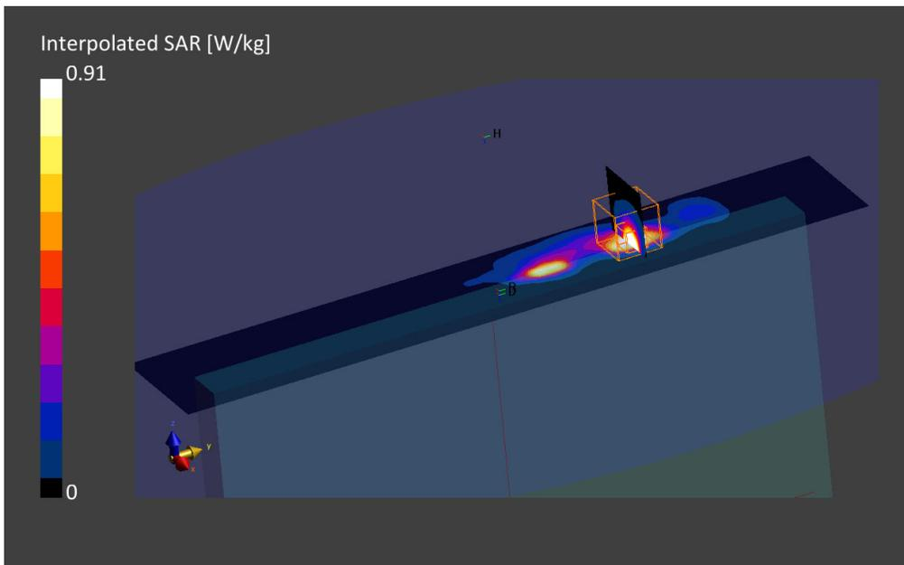
**13. LTE Band 38, QPSK - 20MHz, CH38000, Bottom Edge**
