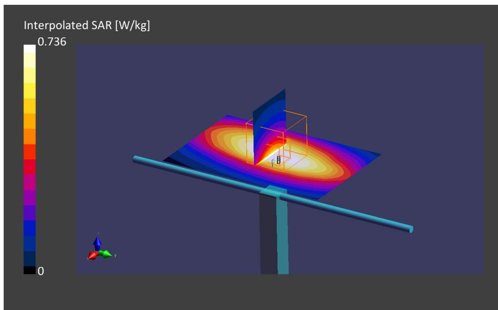
**21. System Check Body Liquid 835MHz – 2022-05-16**
