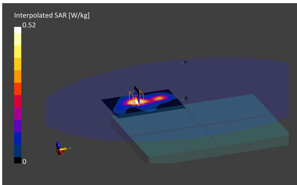
**6. LTE Band 12, QPSK - 10MHz, CH23095, Bottom Edge**
