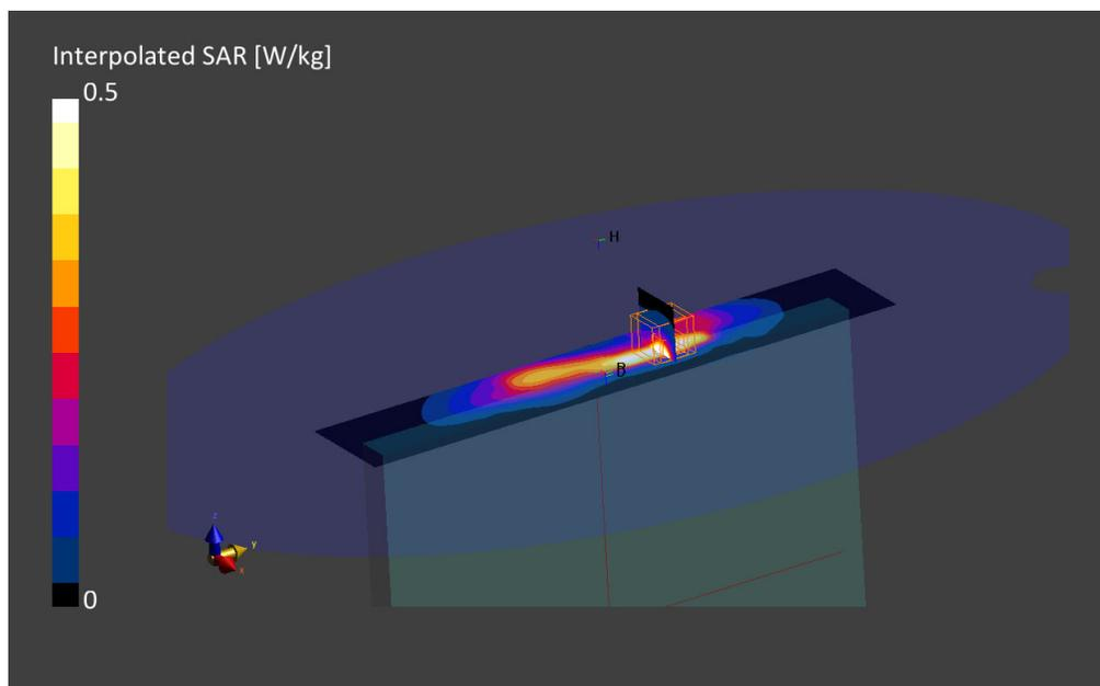
**8. LTE Band 14, QPSK - 10MHz, CH23330, Bottom edge**
