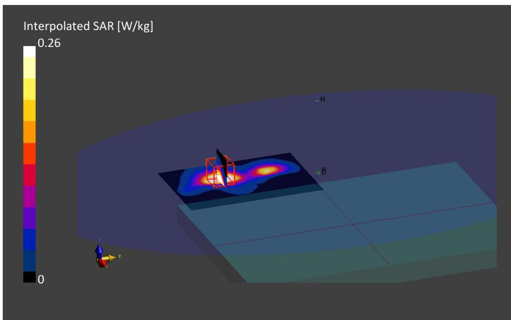
**15. LTE Band 48, QPSK - 20MHz, CH55990, Bottom Edge**
