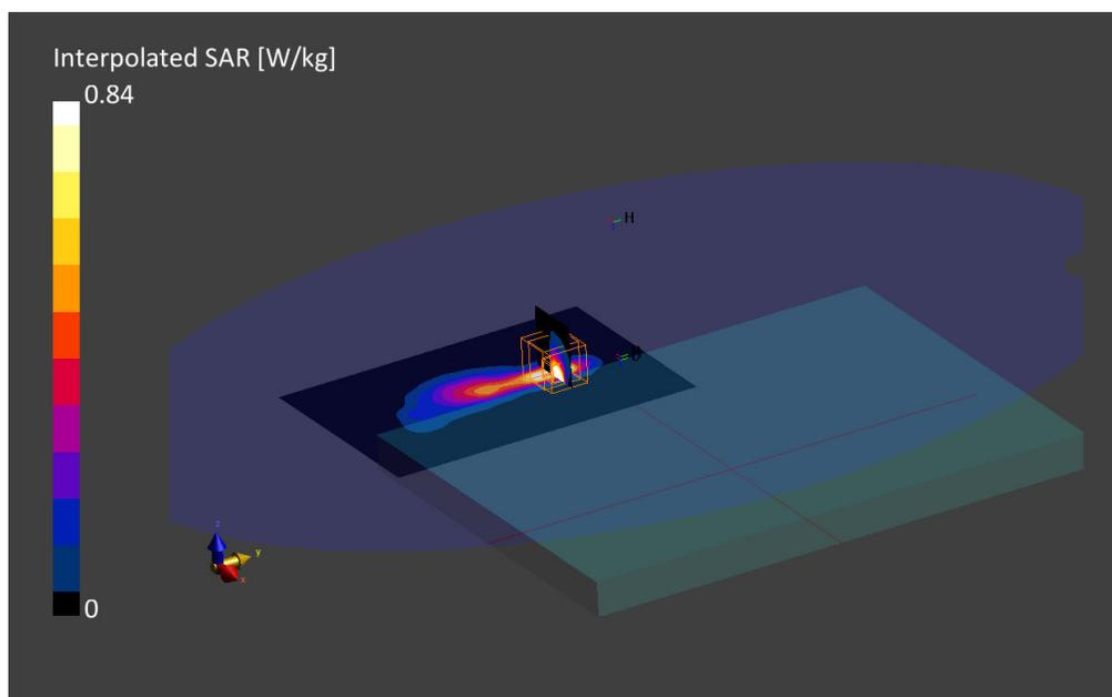
**11. LTE Band 26, QPSK - 15MHz, CH26865, Bottom Edge**
