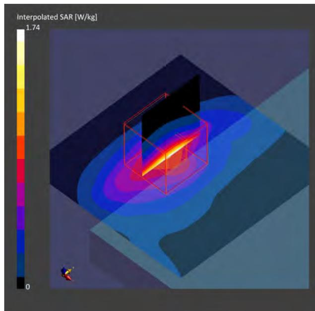
**12. LTE Band 41, QPSK - 20MHz, CH40620, Antenna 8**
