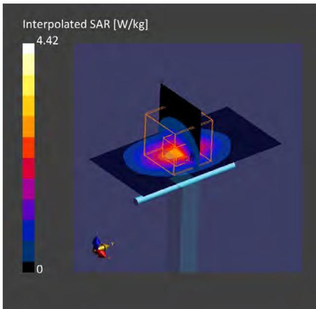
**32. System Check Body Liquid 2600MHz – 2021-12-20 – System 2**
