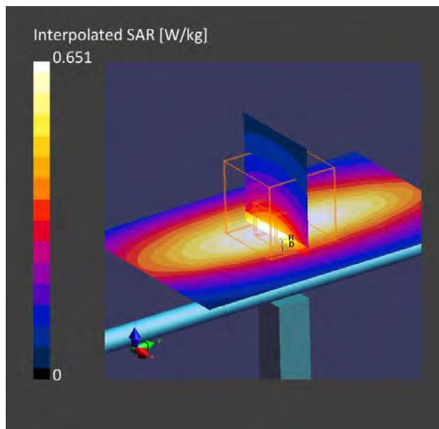
**24. System Check Body Liquid 835MHz – 2021-12-17 – System 2**
