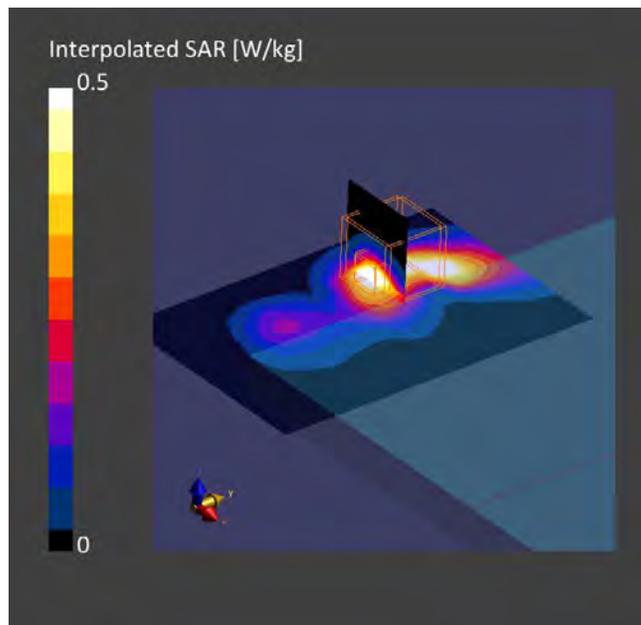
**23. System Check Body Liquid 750MHz – 2021-12-17 – System 2**
