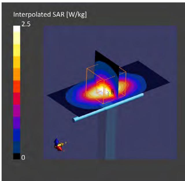
**30. System Check Body Liquid 2300MHz – 2021-12-21 – System 2**
