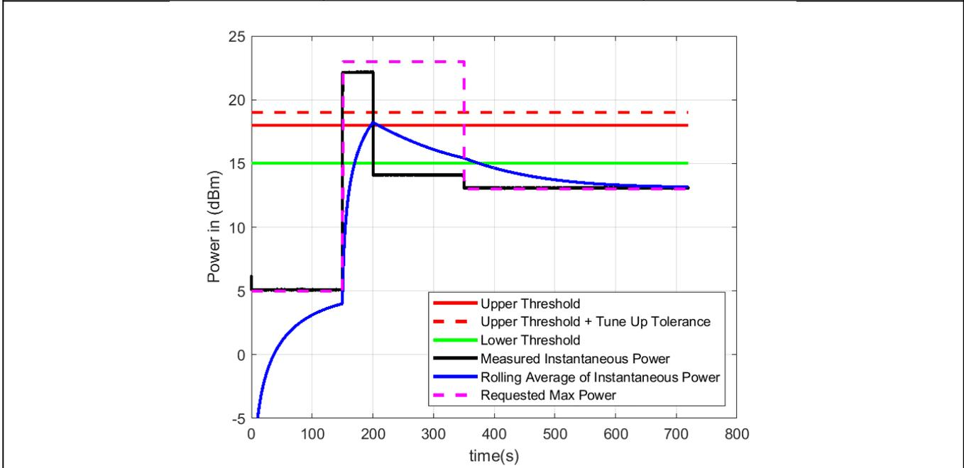
**Case #2: Sequence 2 - LTE Band 2 – Max Power 23 dBm – Roll Period 100 sec – Check Period 0.05 sec**
