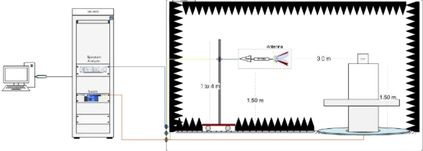
Radiated Setup 18 GHz – 40 GHz (Receiver tests)
