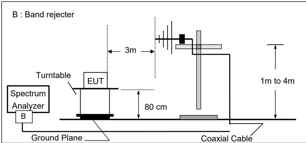
Radiated Emission Test Set-UP Frequency Over 1 GHz
