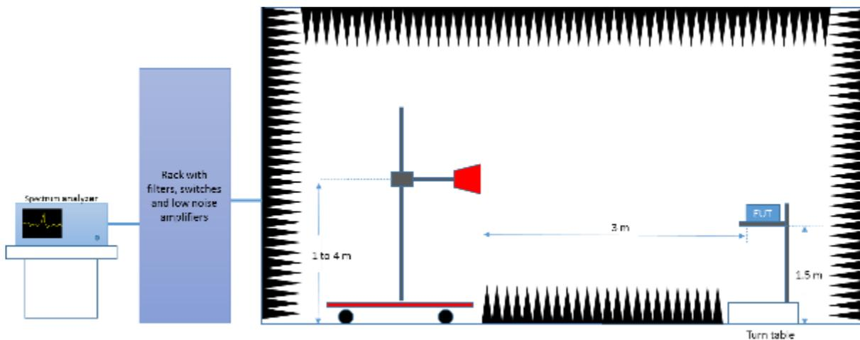
*Radiated Setup Frequency range 18 GHz to 40 GHz*
