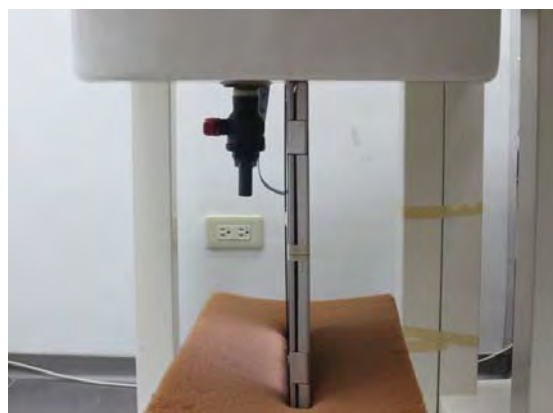
Fig.6 EUT Right side to flat phantom
