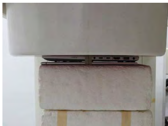
Fig.3 EUT Back side to flat phantom
