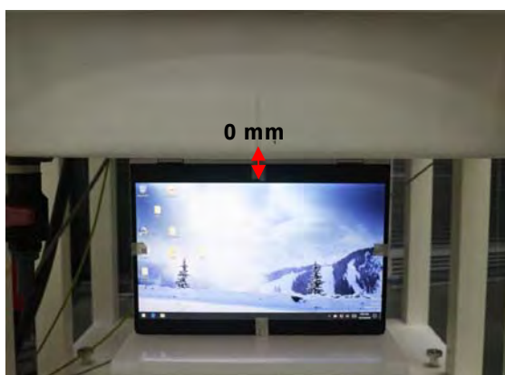
Fig.5 EUT Bottom side to flat phantom
