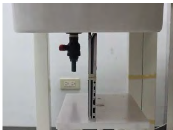
Fig.4 EUT Top side to flat phantom
