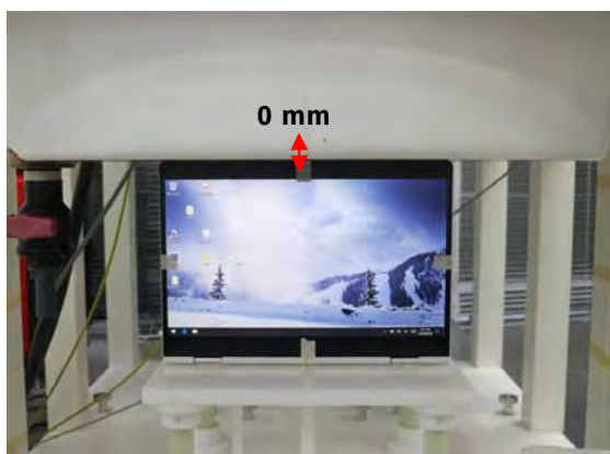
Fig.4 EUT Top side to flat phantom
