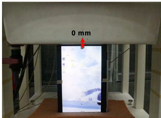
Fig.6 EUT Right side to flat phantom
