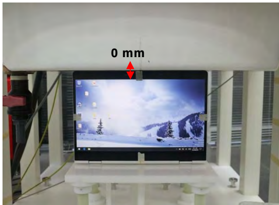
Fig.4 EUT Top side to flat phantom
