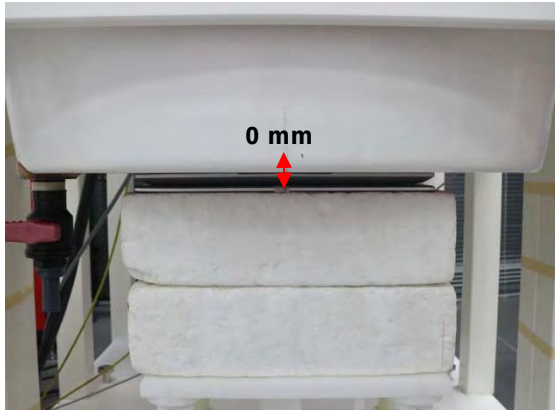
Fig.3 EUT Back side to flat phantom
