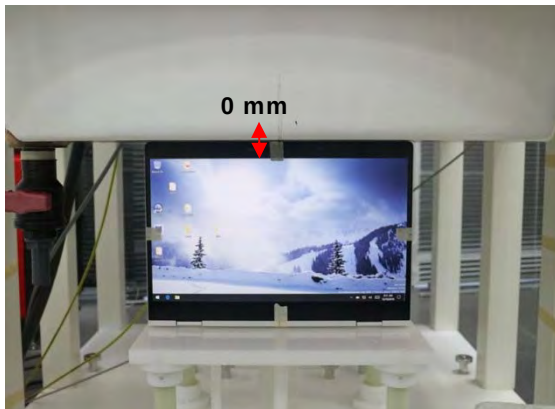
Fig.4 EUT Top side to flat phantom
