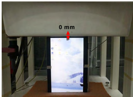
Fig.6 EUT Right side to flat phantom
