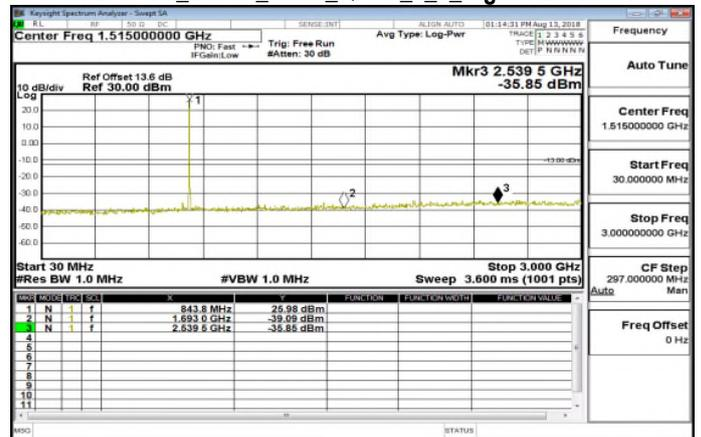
30MHz~3GHz Band5 5MHz QPSK 1 0 MidCH20525-836.5
