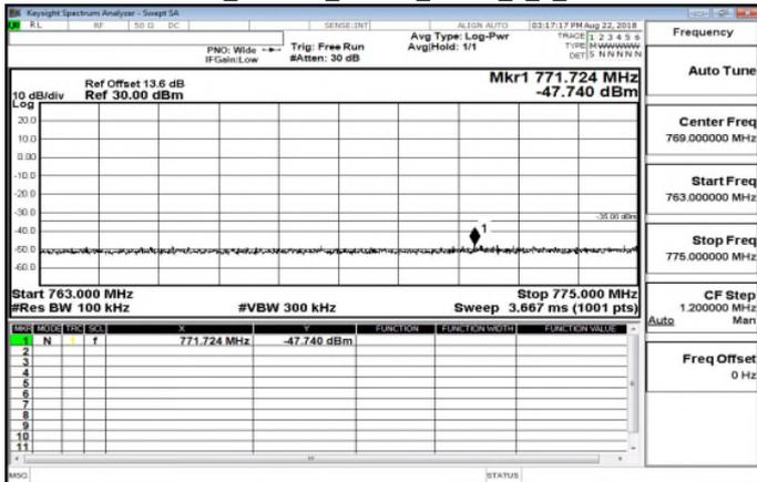
769MHz~775MHz\_Band14\_5MHz\_QPSK\_1\_0\_Full RB 1-Mid
