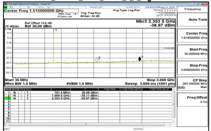
30MHz~3GHz Band13 5MHz QPSK 1 0 MidCH23230-782
