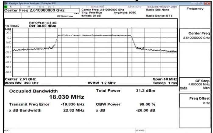
Band38 20MHz 16QAM 100\_0\_LowCH37850-2580
