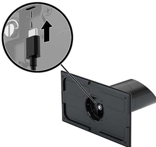
5. Place the I/O connectivity base onto the bottom of the dock's stability base (1), and then tighten the four screws on the underside of the I/O connectivity base (2) to secure the I/O connectivity base to the dock. Be sure that the USB Type-C power cable is routed through the gap between the back of the I/O connectivity base and the dock's column.
