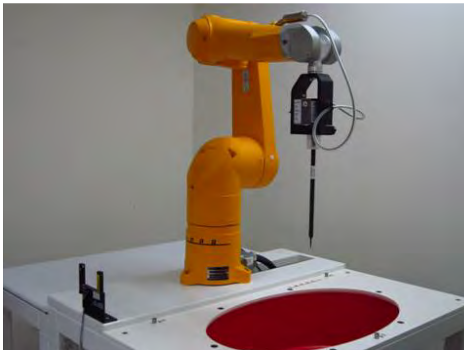
Fig.1 Photograph of the SAR measurement system
