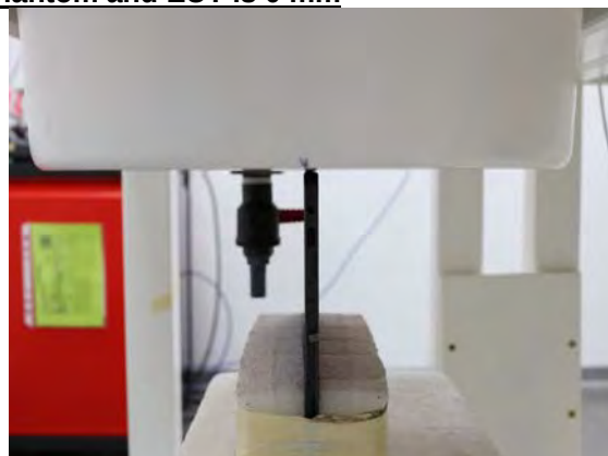
Fig.5 EUT Top side to flat phantom
