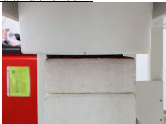
Fig.3 EUT Back side to flat phantom
