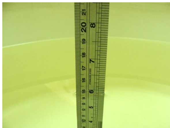
Fig 6.2 Photo of Liquid Height for Body SAR
