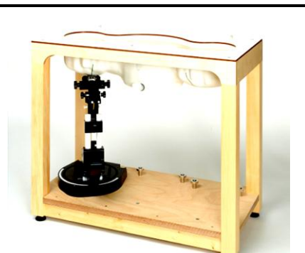
Fig 5.9 Photo of SAM Phantom
