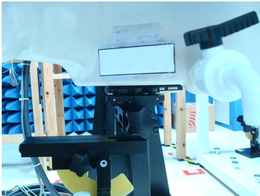
Figure 32. Body SAR Test Setup (Flat Section) _ 0 mm separation
